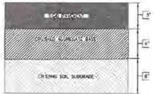
LIGHT DUTY FLEXIBLE PAVEMENT DETAIL ② NOT TO SCALE
