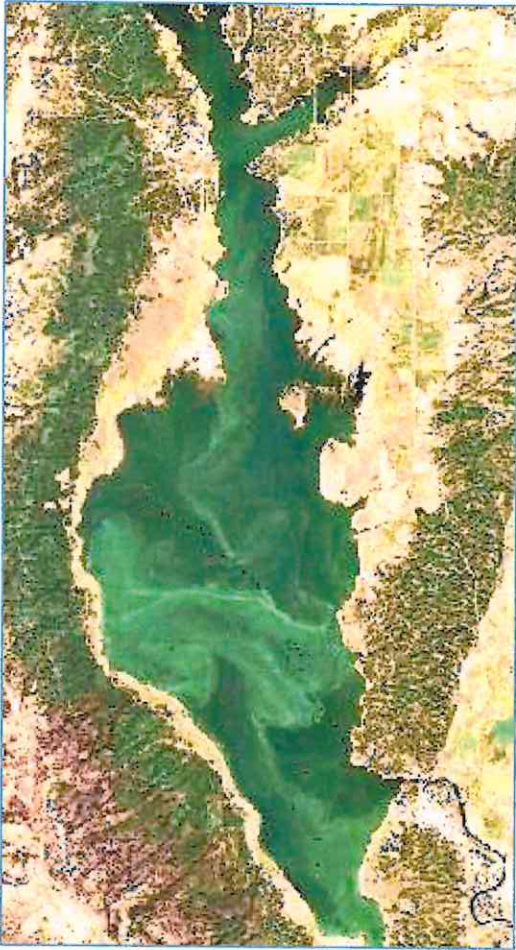
Figure 4; September 30, 2022 Harmful Algae Bloom viewed from Sentinel2 satellite. The brilliant green streaks and swirls that you see are caused for the most part by a bloom of toxic producing cyanobacteria called Dolichospermum . Other toxic producing cyanobacteria like Aphanizomenon , Woronichinia , and Microcystis are also present. Consider the cumulative water quality consequences and need for permanent BMPs before deciding.
