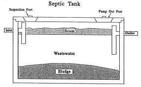
Tees, or baffles, are provided at the tank's inlet and outlet pipes. The inlet tee slows the incoming wastes and reduces disturbance of the settled sludge. The outlet tee keeps the solids and scum in the tank. As new wastewater enters the tank through the inlet tee, an equal amount of wastewater is pushed out of the tank through the outlet tee. The effluent that leaves the tank has been partially treated but still contains disease-causing bacteria and other pollutants.
