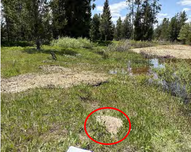
Photo 9: Looking at STP4 along the site's western border, located 3-5 feet upslope from STP3. The soil matrix was 95% 10YR 3/3 and 5% 10YR 4/6 coated sand grains in the first 8 inches. From 8-12 inches the soil was a silty loam with a 10YR 3/1 matrix and 100% 10YR 6/3 from 12-18 inches. STP4 did not pass the dominance test for hydrophytic vegetation or have hydric soils. Therefore, STP4 occurs in an upland.
