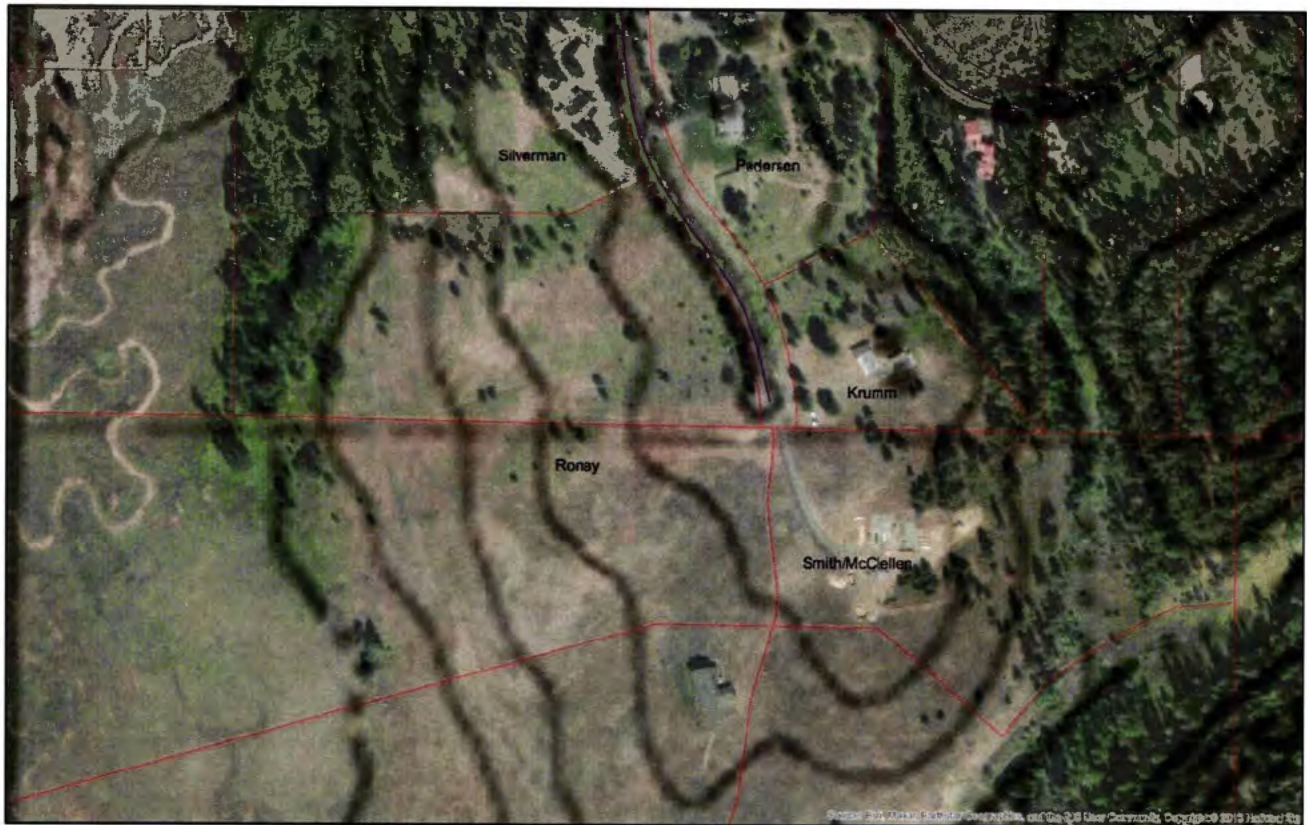
Figure 1. Topographic map created from Valley County GIS website with topographic overlay. Contour interval is 20 feet. The figure shows that Flicker Rd runs south down a broad ridge with drainage to the east and west. This ridge terminates in a broad knoll in the northwest corner of the Smith/McClellan property.
