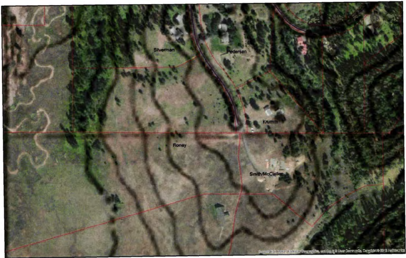
Figure 1. Topographic map created from Valley County GIS website with topographic overlay. Contour interval is 20 feet. The figure shows that Flicker Rd runs south down a broad ridge with drainage to the east and west. This ridge terminates in a broad knoll in the northwest corner of the Smith/McClellen property.
