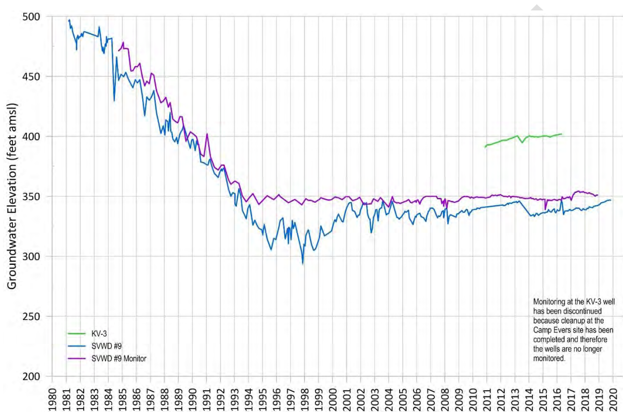
Figure 14. Monterey Formation Hydrographs for Monitoring Wells
